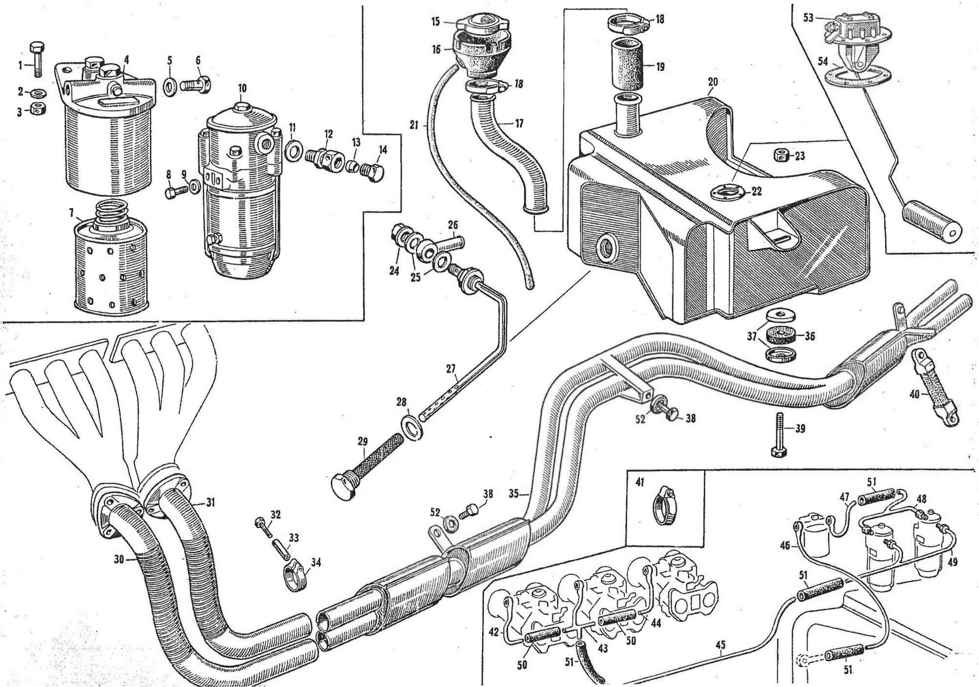
Table 11 - Exhaust manifold and fuel tank
