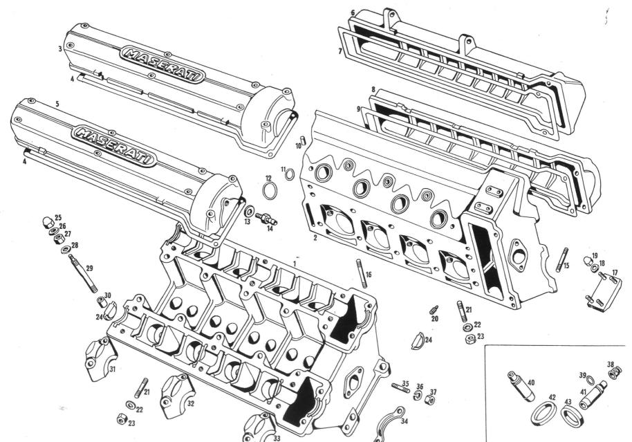
Tavola 1 - Teste cilindri Table 1 - Cylinder heads Tableau 1 - Culasses Tafel 1 - Zylinder Köpfe
