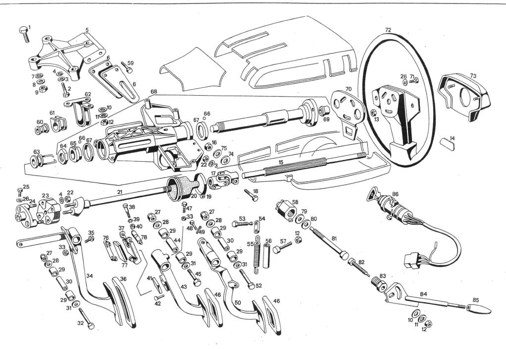
Tavola 18 - Guida e pedaliera Table 18 - Steering parts pedals Tableau 18 - Direction pedalier Tafel 18 - Lenksaule pedale
